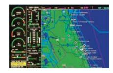
Multi-Function Flight Display (MFD) In the center of the panel, engine data, charts, traffic, weather, flight plans, menus and more are displayed on the large format, high-resolution, 15" display. Garmin's highly-respected user-friendly interface makes the MFD simple to navigate and puts a wealth of information at your fingertips.
